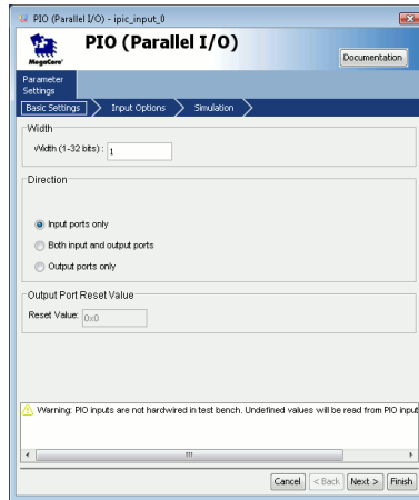
Figure 3.4: Input part of the Interprocessor Interrupt. The Figure shows the Avalon PIO basic settings.
